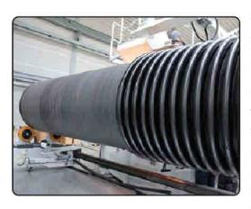
In the larger diameterrange of 800 mm and above what are known as shuttle corrugators are increasingly employed where a small number of moulds are moved back and forth on rails. For instance, in shuttle-type corrugators the corrugator is fed by one or two single screw extruders, usually equipped with barrier screw and grooved feed bush in order to achieve high output of the ployolefin material. If PVC from dry blend is processed, counter-rotationg twin screw extruders are employed.
